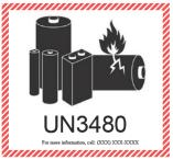
Lithium Battery Handling Marking
